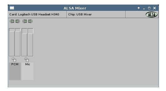
To select a USB Headset as the default audio device, boot TLXOS, plug the Headset into a USB port, enter Ctrl-Alt-t to open an xterm, enter alsamixer which launches the alsamixer audio app, press F6 to select the default Audio device as the USB Headset, then press F3 to select the Playback volume, use the up and down arrow keys to increase or reduce the Headphone volume.
