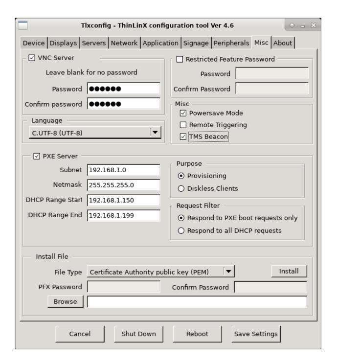
The Misc Tab is used to configure the following,
