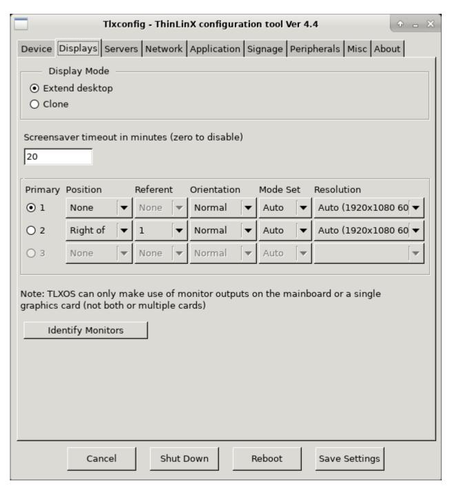
After making any changes click on **Save settings**, you must also do this before pressing the Identify Monitors Tab. In the case of the RPi you will need to reboot before any changes take effect
