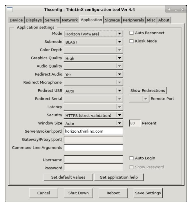
The RPi version of TLXOS only supports Blast (H264) mode as it needs to use the H264 Hardware decoder to display high performance Desktops.
