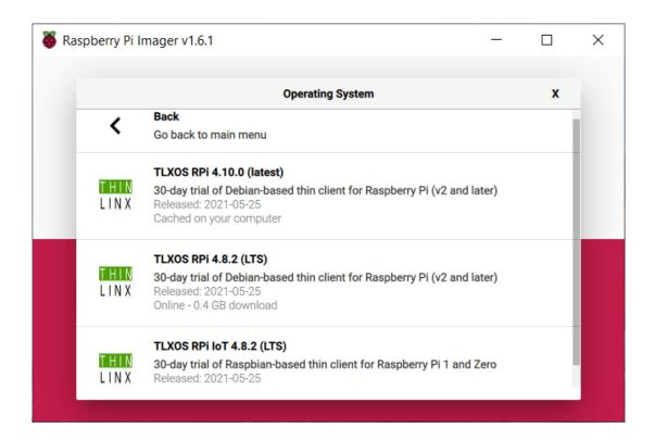
If instead of using the new Raspberry Pi Imager you have installed TLXOS using NOOBS over a WiFi Network and you wish to continue using WiFi once TLXOS has booted for the first time, you will need to configure the WiFi using the local Tlxconfig configuration menu changing the default WPA / WPA2 personal to DIY (use wpa\_supplicant.conf)
