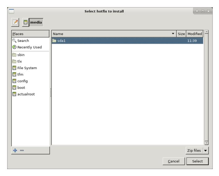
All other files are installed via Tlxconfig menu -> Misc Tab -> Install File dialog section Insert the USB stick into the TLXOS device, select the File Type from the drop down menu, click on Browse, select sda1, select the file to install, click on the Install button
